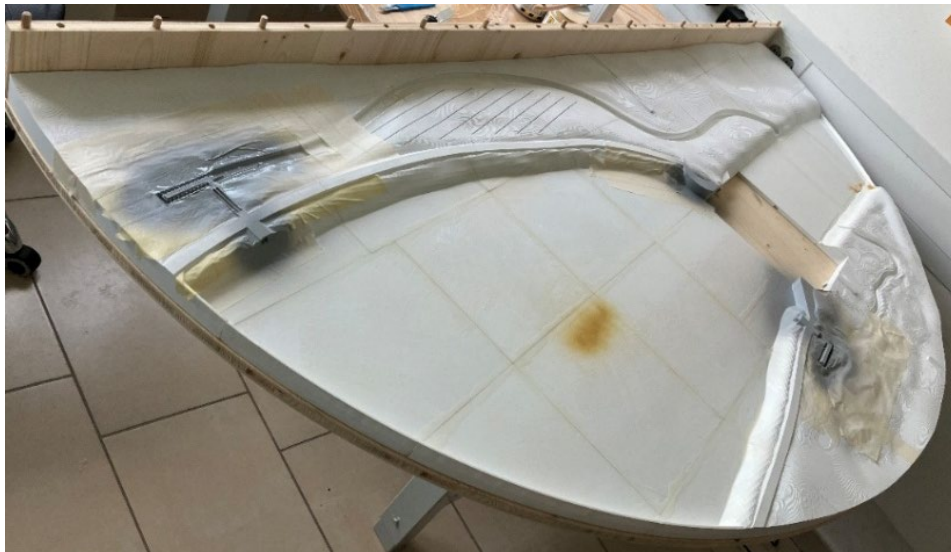
Figure 2: Combined parts that were filled with filler and sanded.
