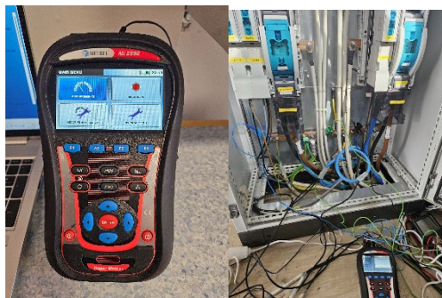
Figure 2: Measuring equipment and the setup: (a) Metrel MI 2892 Power Master Measuring instrument; (b) Connection setup at the point of common coupling (PCC) at the main distribution board.
