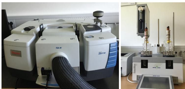
Figure 2: Thermo scientific TGA-IR and Nicolet iS50 FTIR (left), Mettler Toledo EasyMax 102 (right)
