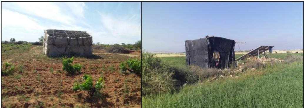
Figure 17: The Aacha Housing is Built with Mixed Fragile Materials in Doukkala East.
