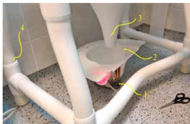
Figure 6. The Dorado KT system is shown with a toilet stand 4 and funnel 3 . Our specimen container 2 is placed on the weight cell 1 of the Dorado KT system.
