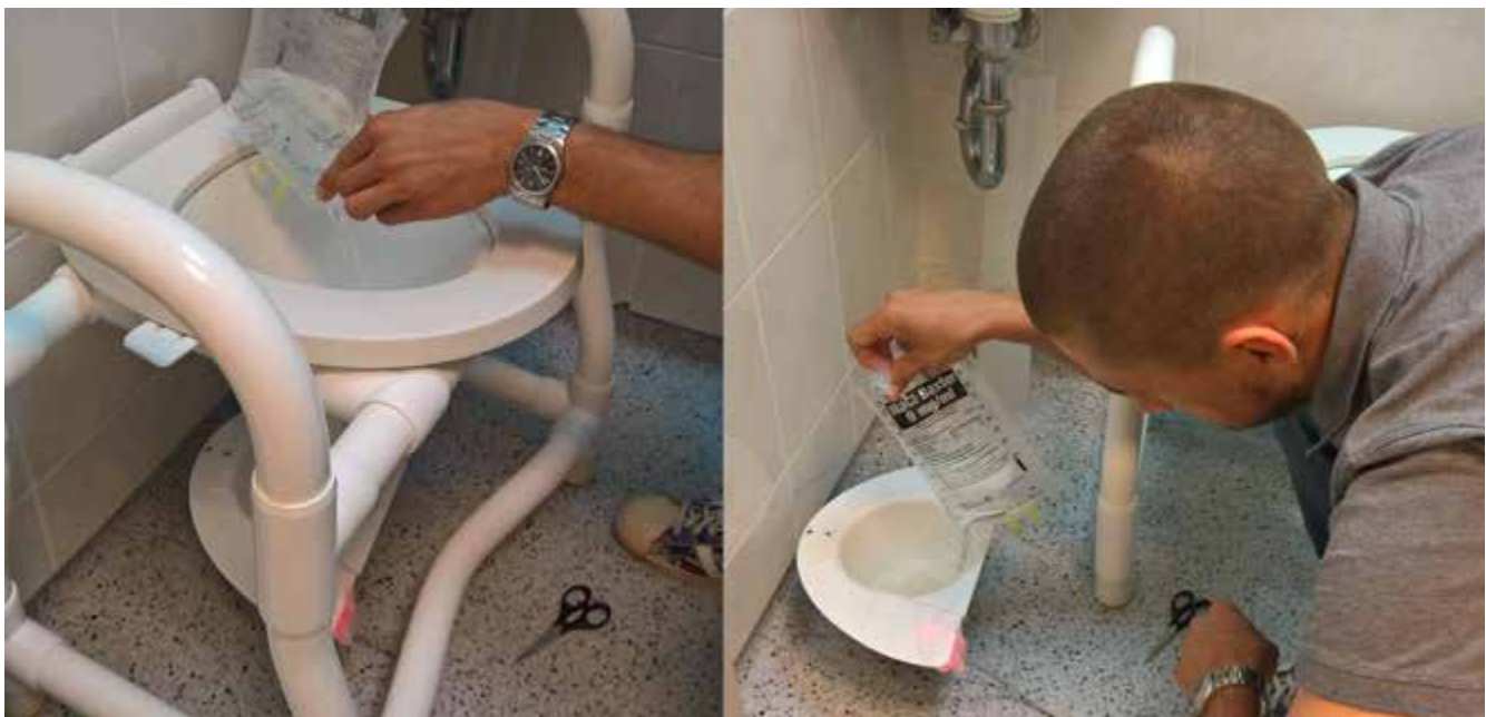
Figure 7. The Dorado KT system is shown equipped with a simulated toilet stand, funnel, and weight cell. The novel capacitive device is shown (left) with the specimen container positioned on the weight cell of the Dorado KT system (right) as it was for the comparative evaluation.
