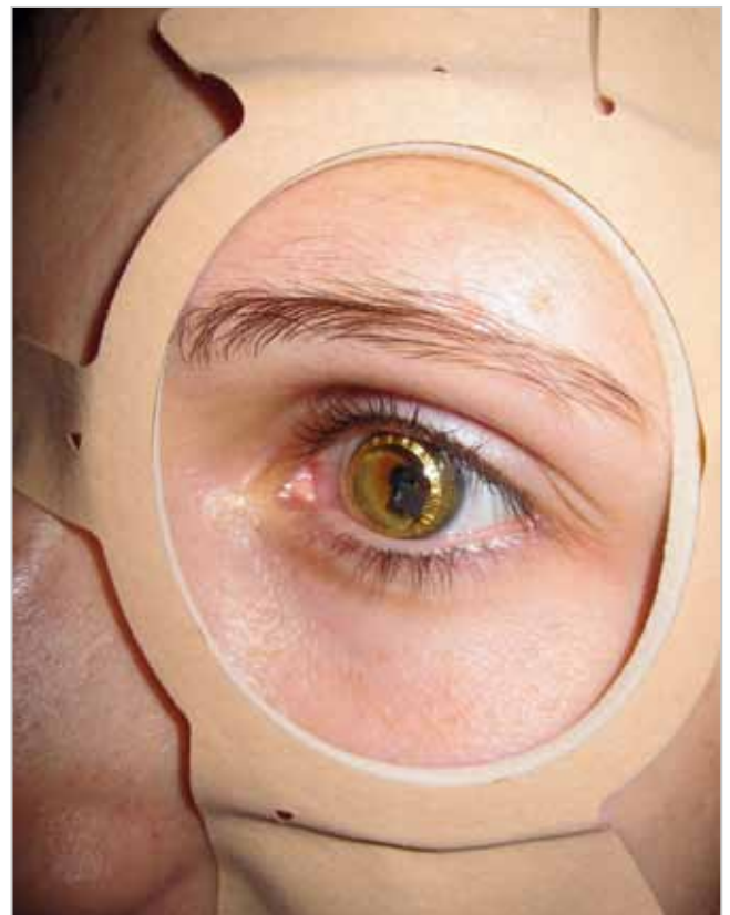
Figure 1. Sensor contact lens in the left eye, the square microprocessor and the golden antenna are easily visible. Around the orbita a second antenna for data transfer is placed.
