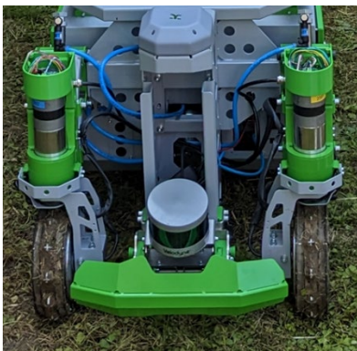
Figure 2: The front of the FarmBeast robot with a mounted Velodyne VLP-16 multichannel LiDAR
